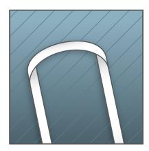
Apply heat tape in back-andforth runs as shown. Leave end loops with adhesive side up.
