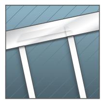
Apply Heat Transfer Tape across end loops and roll down firmly.
